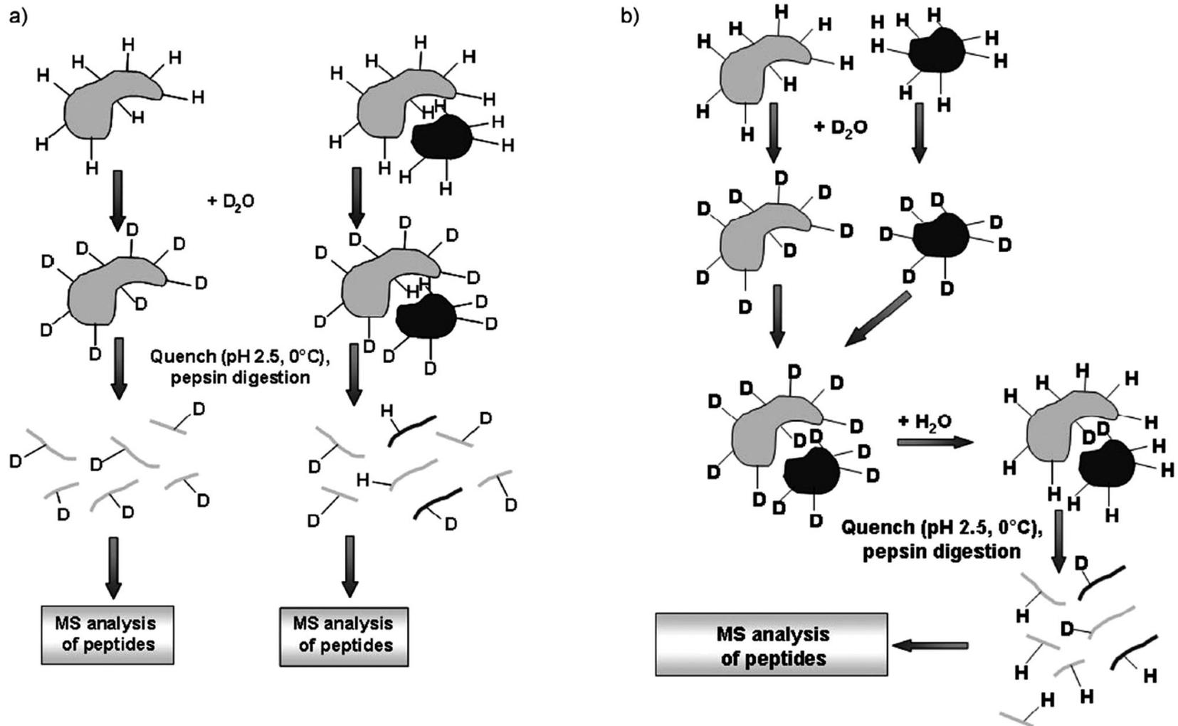
**Fig. 9** Scheme of on- and off-exchange approaches used in HDX experiments. Reproduced from A. Sinz, 2007<sup>5</sup> with permission from John Wiley and Sons.
