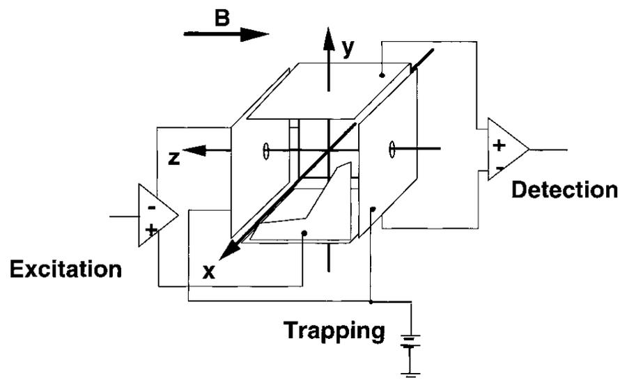
**FIGURE 7.** Incoherent ion cyclotron orbital motion (top left) is converted to coherent (and, therefore, detectable) motion (top right) by the application of a rotating electric field, which rotates in the same sense and at the ICR frequency of the ions of a given  $m/z$  value. The electronic circuitry is shown in the bottom diagram.
